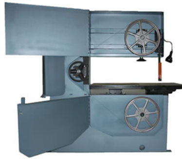
DT1340 with top and bottom doors open.
